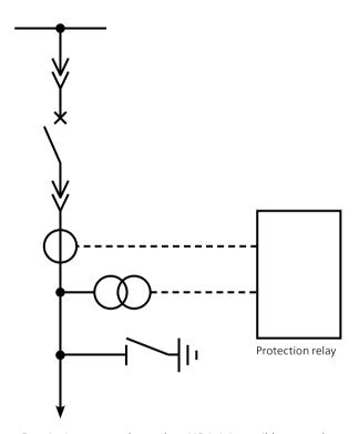
For tripping currents lower than 110 A, it is possible to test the complete chain from the primary site of the current transformer to the contacts of the circuit breakers.
