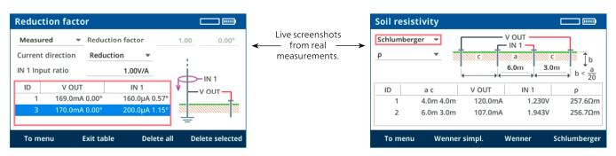
Integrated measurement and calculation of the current reduction factor.
